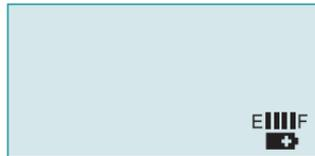
*Figure 2-27 Battery Power Indicator*
