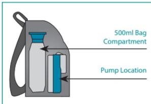
Figure 6-8 Super-Mini Backpack (Cutaway View of Internal Compartments)
