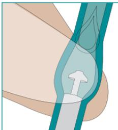
Figure 2-6 Tubing Segment Being Pinched
