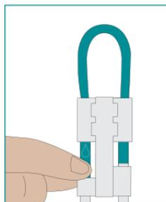
Figure 2-5 Pincement de la tubulure
