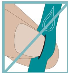
Figure 2-7 Tubing Segment Being Punctured by Fingernail
