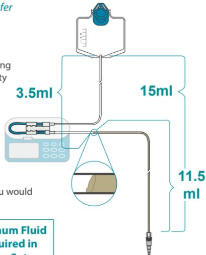
Figure 9-1 Disposable Set Residual Fluid
