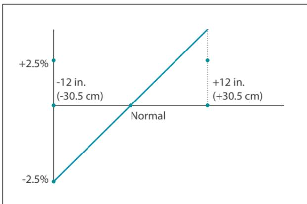
Figure 8-1 Head Height Effect on Accuracy
