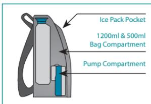
Figure 6-13 Backpack (Cutaway View of Internal Compartments)
