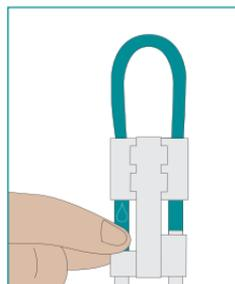
Figure 2-5 Pinch Tubing
