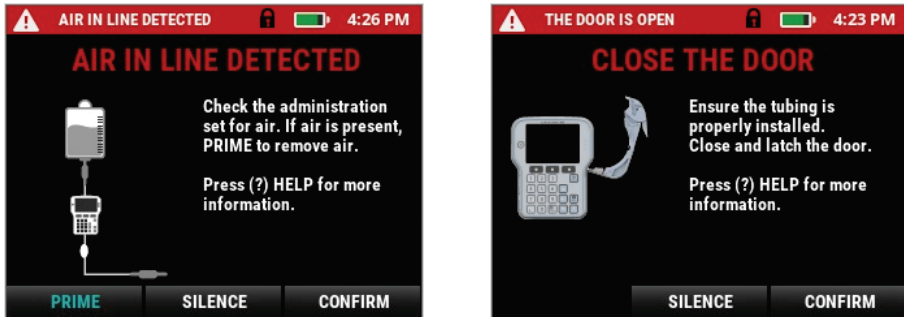
Figure 16: High Priority Alarm Screen Examples
